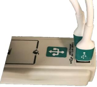
A power strip is shown with a green USB port. A white charging cord with a green USB-A connector is plugged into the port. The power strip is labeled "USB Charge" and "W750 (MAX)".                                                                    |
