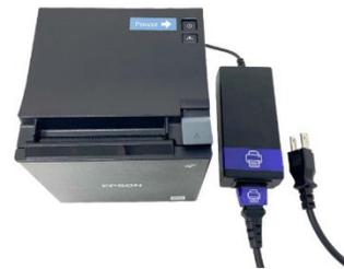
6. Plug the cord with the orange sticker into the back of the ExpressVote Printer above the orange sticker. The flat side of the cord should be facing downwards while the lightning bolt should be facing upwards. Plug the other end of the cord into the power strip.
