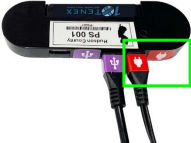
A black ExpressVote printer is shown from a top-down perspective. A red power button is highlighted with a green rectangular box. A purple USB cable is plugged into the front of the device. A label on the printer reads "TENEX Hudson County PS 001". |
